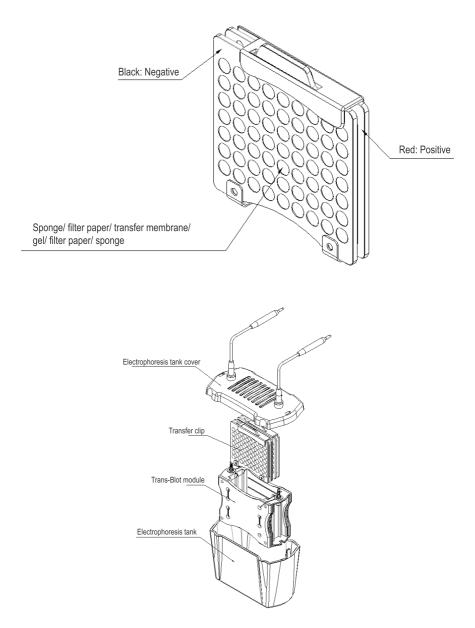
Connect electrophoresis, set transfer conditions: 300mA, constant current for 30min, start film transfer.
